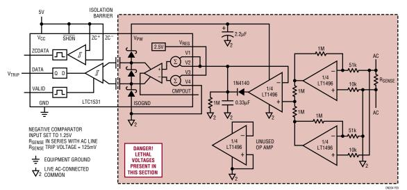
Figure 3. AC Line Overcurrent Detect
