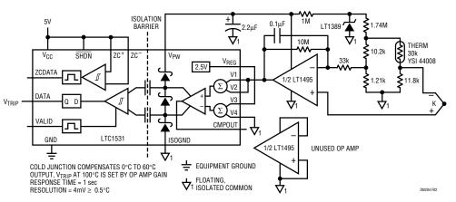
Figure 2. Overtemperature Detect
